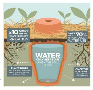
Osmosis theoretically will continue until the concentration is equal on both sides. The beauty of this system is that if it rains, the amount of water molecules on the soil side of the jar is higher, so osmosis will slow or even stop until the soil starts to dry out and then osmosis will begin again. This means it is impossible to overwater or waste water.
